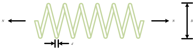
Fig. 18. The schematic view of the tension/compression spring design problem.
