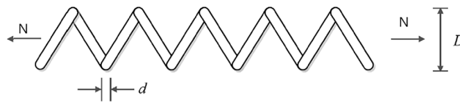
Fig. 14. Schematic of tension/compression spring design.
